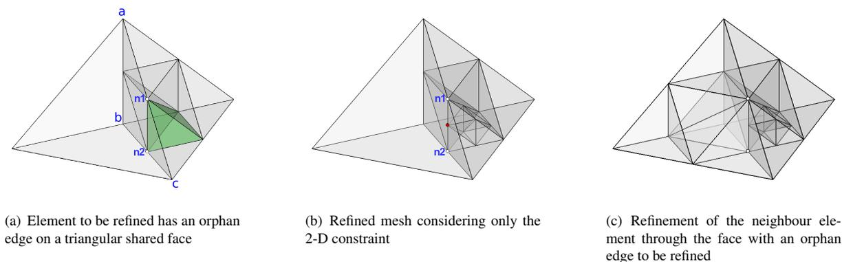
Figure 2: Refinement constraint for 3-D meshes - Orphan edge case.
