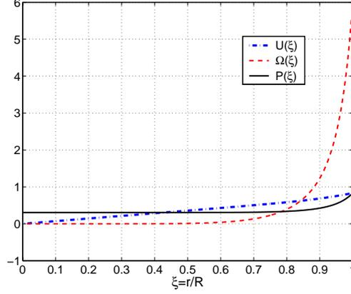
Figure 3: Self-similar profiles for the spherical blast wave problem ( $\gamma = 1.4$ ).
