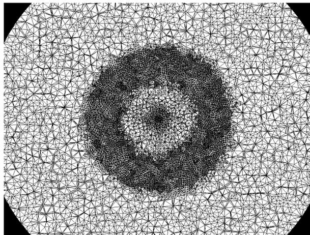
Figure 6: Adapted mesh on a plane of symmetry at time  $t = 0.645ms$ .
