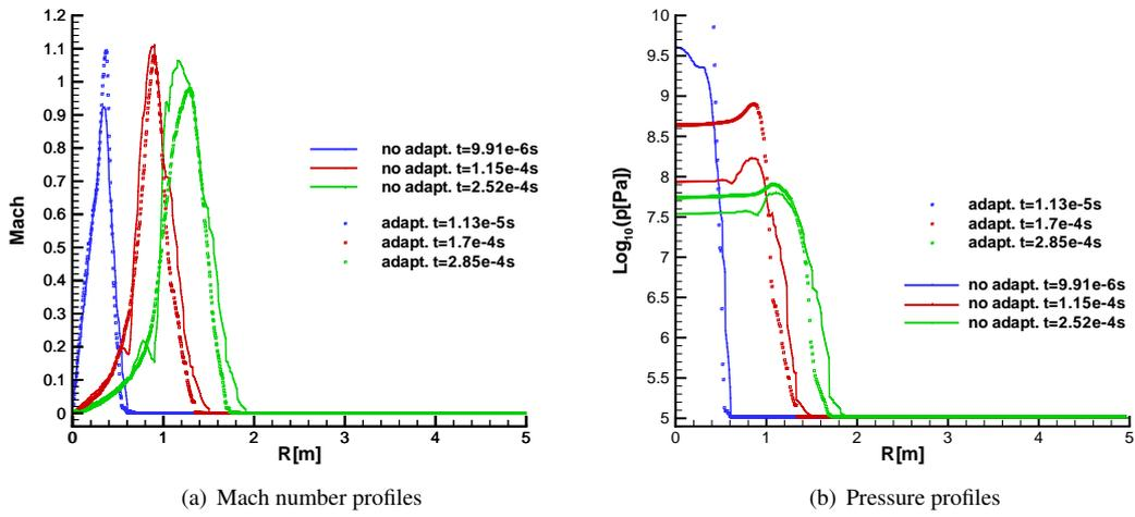
Figure 5: Time evolution of the flow field within the blast wave.
