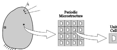
Figure 2: Representation of a composite material made of a periodic microstructure
