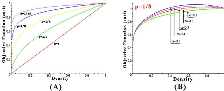
Figure 9: Different penalizations for equation (8): (A) varying  $p$  ( $\alpha=0$ ) and; (B) fixed  $p$  ( $=1/8$ ) and different values for  $\alpha$
