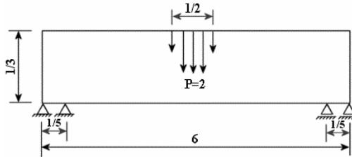
Figure 10: MBB beam under flexion (SI units)
