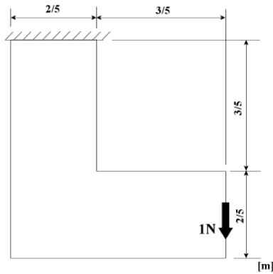
Figure 17: Geometry and boundary conditions for the L-shape beam
