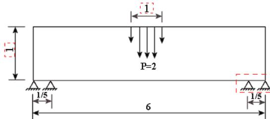
Figure 12: Another problem using MBB beam under flexion (SI units)
