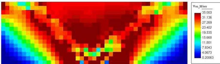
Figure 16: Stress field for the optimized problem.  $\sigma_{\max}=35 \text{ N/m}^2$
