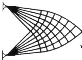
Figure 1: One load case Michell-like truss structure. It is the best possible truss for this specific load case. Notice that the bars crossing themselves forming  $90^\circ$ . This is an unstable structure for any other type of loads
