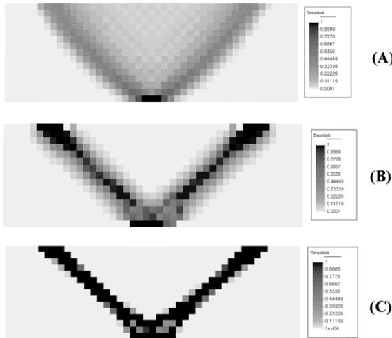
Figure 15: Final results for  $\varepsilon=10^{-7}$ ; (A)  $p=1, \alpha=0$ ; (B)  $p=1/8, \alpha=0$ ; and (C)  $p=1/8, \alpha=0.3$
