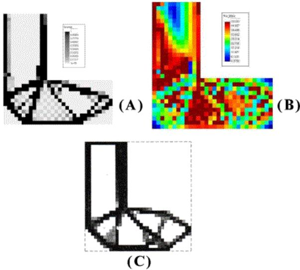
Figure 18: (A) Final topology for  $\varepsilon=10^{-8}$ ,  $p=1/8$  and  $\alpha=0.3$ ; (B) stress field,  $\sigma_{\max}=50.5 \text{ N/m}^2$ ; and (C) Similar final topology obtained by Duysinx and Bendsoe<sup>15</sup> (1998) with 9-node quadrilateral elements
