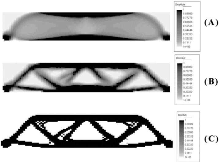
Figure 11: (A) Solution without penalization; (B)  $p=1/8$ ,  $\alpha=0$  and; (C)  $p=1/8$ ,  $\alpha=0.3$
