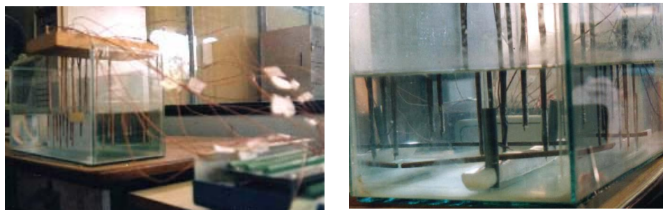
Figure 3. Experimental setup: view of the fixed ice rod and measurement device.
