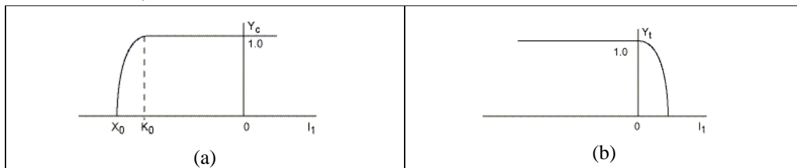
Figure 7: (a) Elliptical compressive cap; (b) Elliptical tensile cap (from Release 11.0 Documentation for ANSYS)
