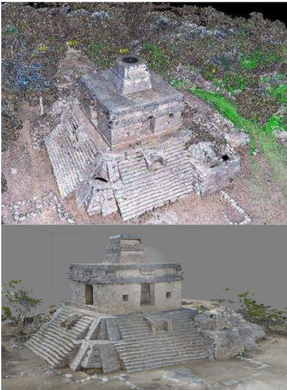
Figure 10: 3D Point-Cloud Model (top) and 3D CRP Model (bottom) of the Temple of the Seven Dolls
