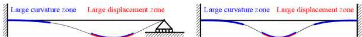
Figure 2: First modal shape of a C-P and a C-C beam.
